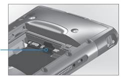
5. Push the flexible card holder back into place, covering the card slots.
